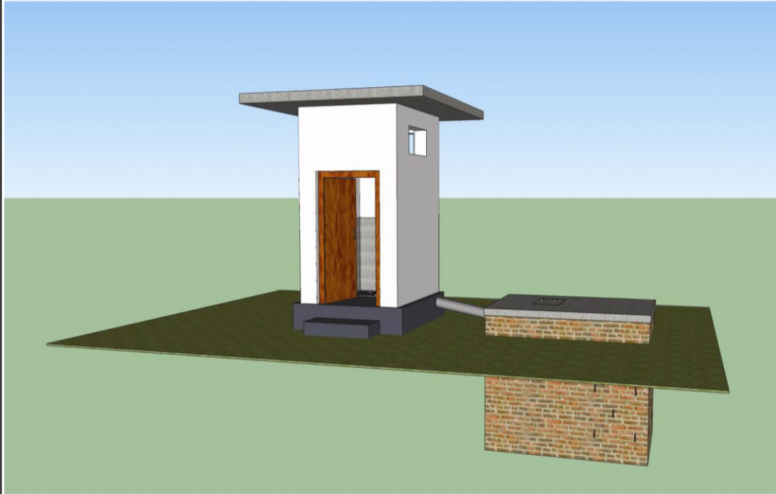
TOILET WITH SEPTIC TANK
